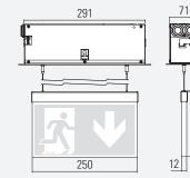
Ceiling cutout: 295 mm x 75 mm Maximum ceiling thickness: 43 mm
