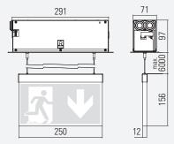
Ceiling cutout: 295 mm x 75 mm Maximum ceiling thickness: 43 mm
