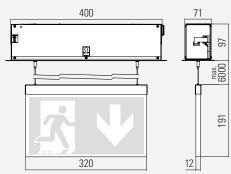
Ceiling cutout: 405 mm x 75 mm Maximum ceiling thickness: 43 mm
