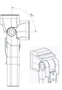
To adjust the light beam to a desired angle, the lamp head can be swivelled in continuous angles from vertical 0° to 30° in front and 90° to the rear.
