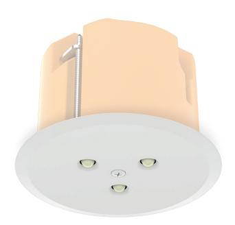
LED emergency luminaire in round design with symmetrical lighting for flush ceiling installation in an existing device junctionbox with standard combination distance of 71 mm in accordance with DIN 49073-1 (deeper version). Suitable for lighting open areas and escape routes in accordance with EN 1838.
